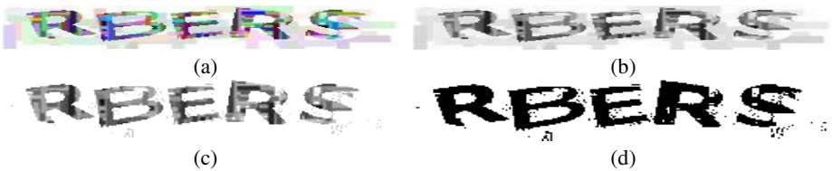
Fig. 7. a) Color Image (b) Grey scale image (c) Color 255 replaced with white (d) Color 133 replaced with black
