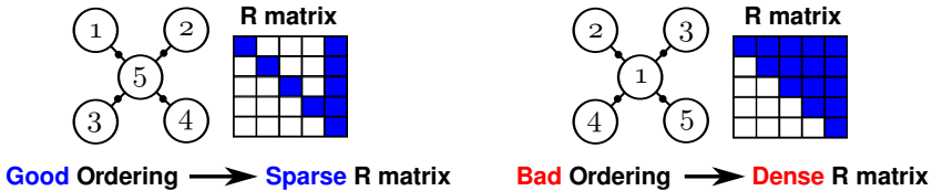
Fig. 4. An illustration of how the elimination ordering affects the sparsity of \mathbf{R} matrix. Suppose we eliminate the leaf vertices first, the \mathbf{R} matrix will be very sparse. Yet if we eliminate the center vertex first, it will introduce a clique over the remaining vertices, and hence the \mathbf{R} matrix becomes very dense, which negatively affects the performance.
