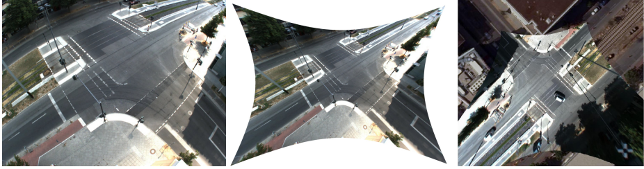
Fig. 6. Original (left), normalized (middle) and transformed image (right)
