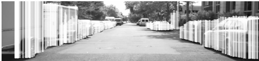
(a) Correct estimation of the environment consisting of static objects. Thus, all Stixels are drawn with a white coloring which denotes a velocity close to zero.
