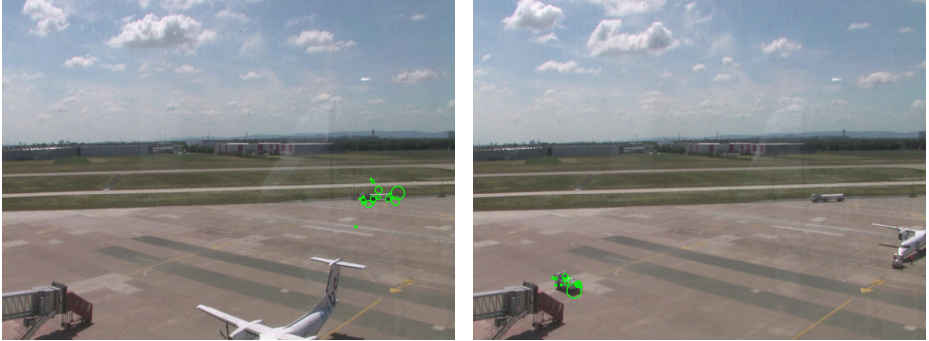
Fig. 7. Motion segmentation of small objects. Compared to the image resolution of 1440 \times 1080 \text{ pel}^2 , the objects are quite small with approximately 110 \times 70 \text{ pel}^2 (left) and 100 \times 100 \text{ pel}^2 (right). Similarly, the number of features (18 and 15, respectively) is only a fraction of the global scene (966 and 891, respectively).
