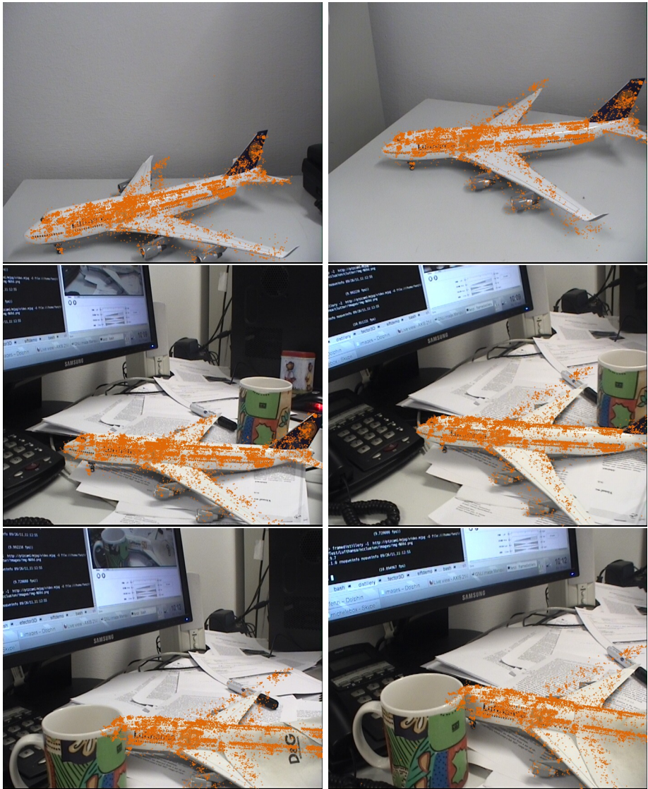
Fig. 13. Example of the 3D tracking of a toy plane. Different situations are presented: blank background, clutter and a combination of clutter and occlusion. The model cloud is reprojected in orange to show the preciseness of the estimated pose.
