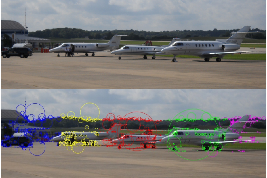
Fig. 11. By spatial feature clustering, the objects in the scene are segmented into five different clusters. This increases the inlier-outlier ratio for each cluster, and permits to avoid mismatches due to objects having a similar appearance, as in the case of the three airplanes.
