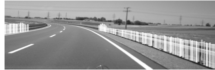
(b) In contrast, successful optical flow computation allows to obtain correct Stixel velocity estimates. The guard rail is covered much better.
