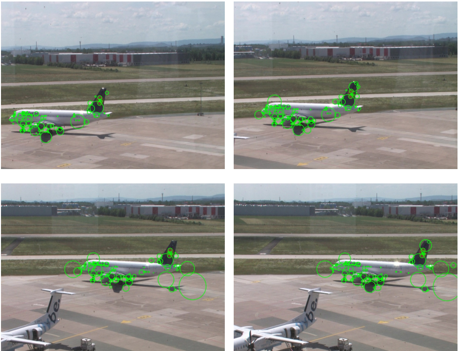
Fig. 8. Motion segmentation under panning and tilting. The four images are taken during a time span of 2 s. As it can be observed, that although the segmented airplane is moving slowly compared to the panning, it is segmented correctly.
