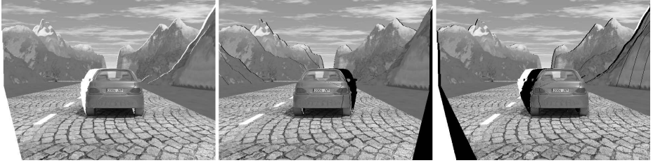
Fig. 4. Different types of occlusions for a horizontal configuration. Left : white pixels indicate occlusion between reference and match camera. Centre : black pixels indicate occlusion between third and reference camera (here: third camera is at position of match camera). Right : combined visualisation where third camera is now left of the reference camera.
