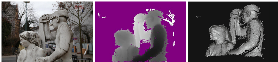
Fig. 1. Left: An input image to Multi-View Stereo reconstruction. Middle: The reconstructed depth map visualized in gray values (white: far, black: near). Right: The triangulated depth map rendered from a slightly different view point.
