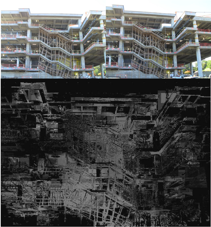
Fig. 10. 3D reconstruction of site construction application
