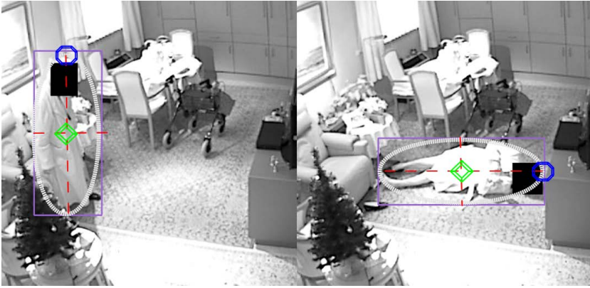
Fig. 7. Extraction of fall features: purple: bounding box, white: bounding ellipse, green: center of gravity, blue: head position (The black box is for privacy reasons)
