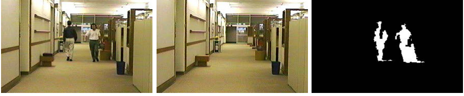
Fig. 2. Background removal using a multivariate background probability. Displayed are input image I_t , the average background \mu , and the foreground mask F . It can be observed, that the shirt of the left person is only partially detected as foreground since it looks similar to the background. Furthermore, shadows on the floor are detected as foreground.
