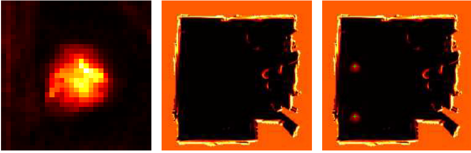
Fig. 4. The occupancy map is generated from combining the human model and the background model. For each set of locations of persons, i.e. a particle, an occupancy map is estimated. Left: Human model. Middle: Background model. Right: Occupancy Map given the hypothetical location of persons (green crosses).
