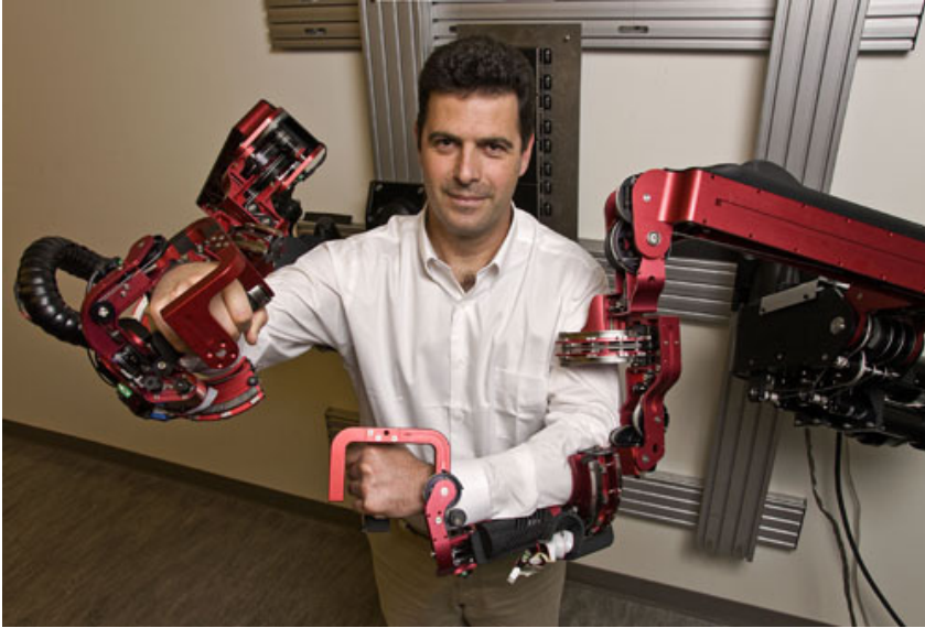
Fig. 1 The upper limb exoskeleton with seven DOFs, supporting 99% of the range of motion required to perform daily activities
