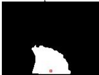
Gray + low-pass + contrast + geometric-mean + threshold
