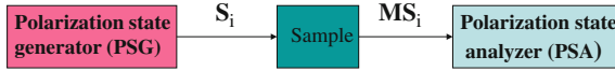
Fig. 2.15 Schematic representation of the optical setup of a general Mueller ellipsometer. The Stokes formalism has been used to represent the polarization properties of light. In the framework of Stokes formalism the optical properties of the PSG, sample and PSA can be represented by matrices
