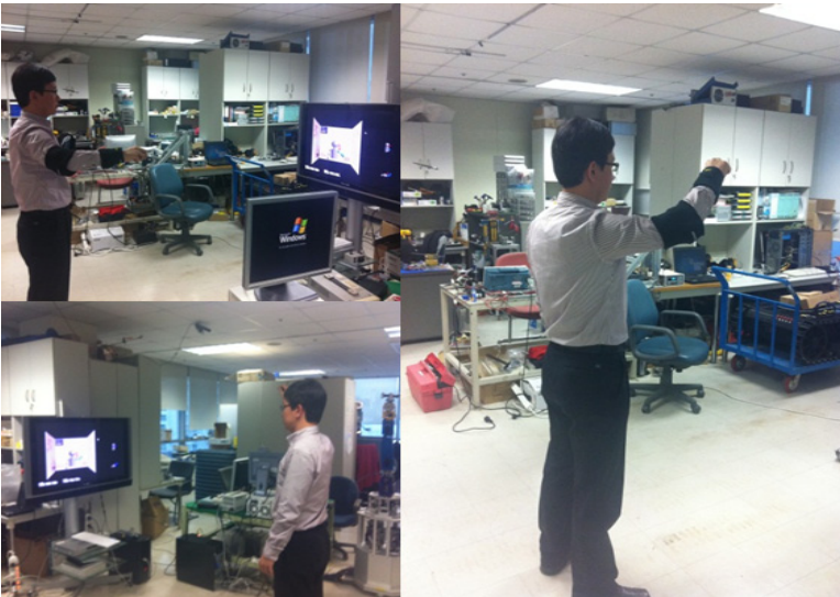
Fig. 1. Two vibrotactile bands are worn on the right arm. Eight actuators are mounted in the vibrotactile band. KINECT sensor for motion capture is attached to ceiling. User motion and desired motion displayed on the monitor.
