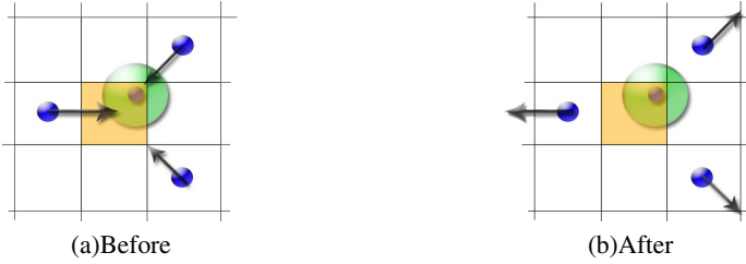
Fig. 7. This figure gives an overview of the translate and collide processes for a fluid cell next to an obstacle
