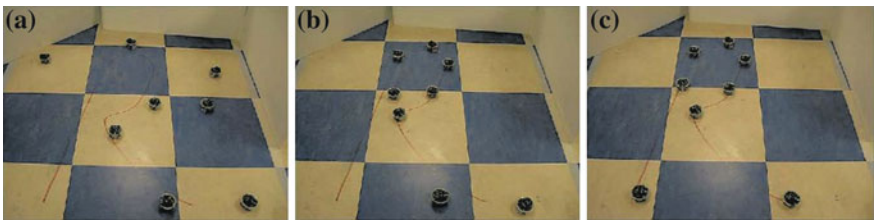
Fig. 3.5 Formation of letter ‘R’ using eight e-puck robots. a t = 0s , b t = 6s , c t = 11s
