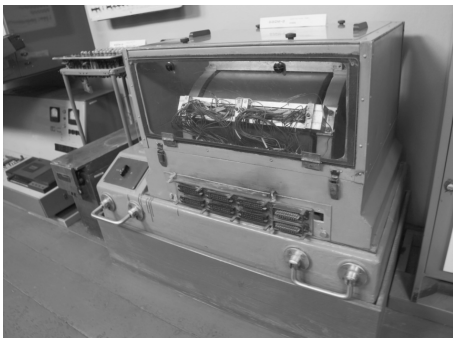
Magnetic DRUM – ‘hard disk’
