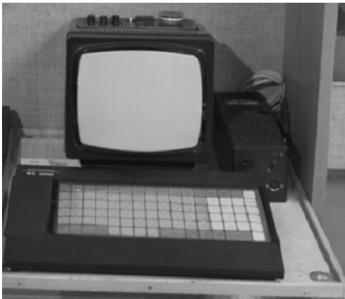
BK-0010 for schools – components: home colour TV, pseudo-membrane keyboard combined with processor and memory
