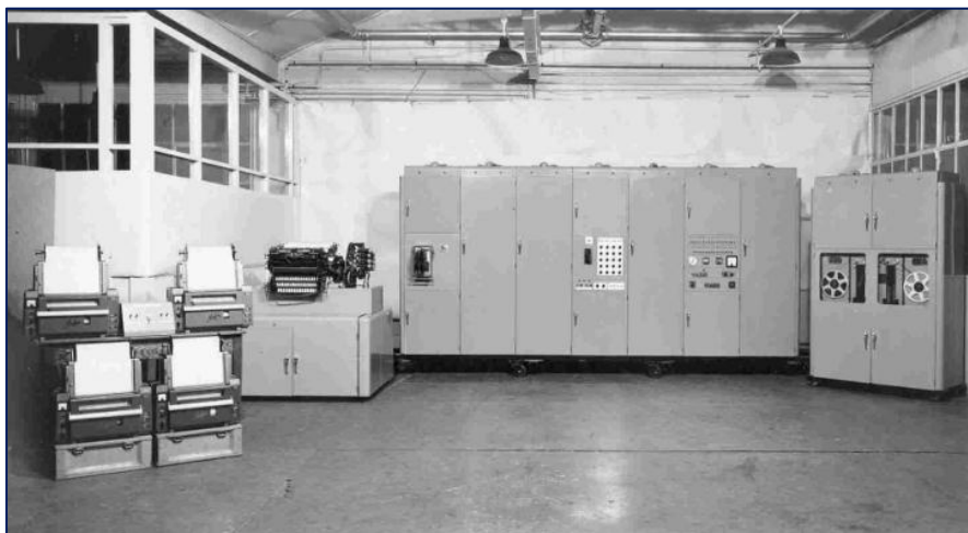
The Elliott 403's Output Converter in the UK in 1955: 4 Mufax plotters, Bull Line printer, Output processor, Magnetic Tape input (from the Elliott's archive at BAE Systems and Telent PLC UK)
