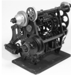
Fig. 4. Electro- mechanical Totalisator: 'Julius Horse Adder', c 1926.
