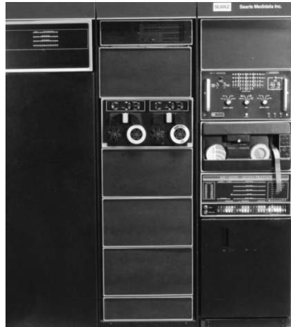
Fig. 14. Searle Medidata Medical Computer based on PDP-8/1
