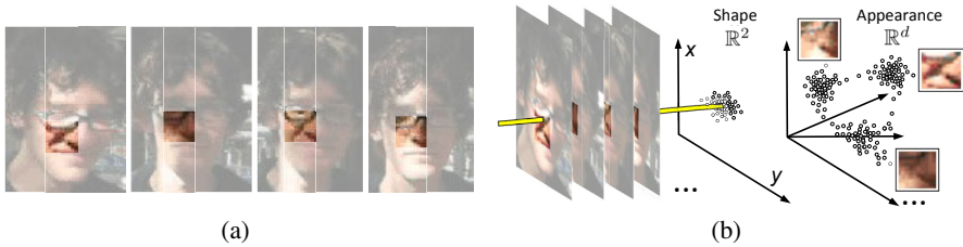
Fig. 1. The weakly aligned multi-instance local features concept in the case of tracking a face. (a): Four frames from the trellis-sequence [3] with highlighted appearance variations in a particular object region susceptible to self-occlusions and shadows. (b): Region representation after weak alignment. Feature locations describing 2D shape in the xy -coordinate system of the object template are shown with their associated appearance descriptors (128D).
