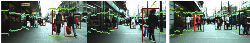
Fig. 6. Some example frames from the result video (see supporting material). Blue lines indicate stixels estimates, boxes mark detected pedestrians.
