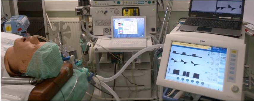
Fig. 4. The current testing environment of the developed CG, showing the Human Patient Simulator and the mechanical ventilator
