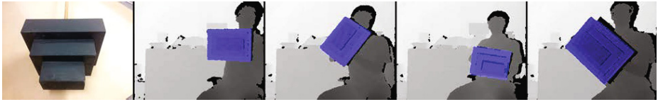
Fig. 5. The leftmost images shows our calibration object, Film strips to the right shows an example sequence that we used for simultaneous calibration and tracking
