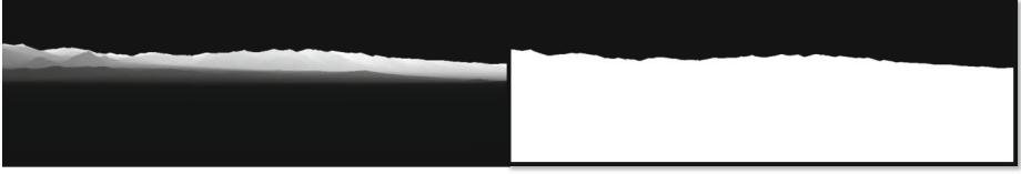
Fig. 2. Example of a rendered depth image and its extracted skyline. To extract the skyline, the system looks at the depth image from top to bottom in each column, and labels as skyline pixel the first pixel with a non-infinite depth.
