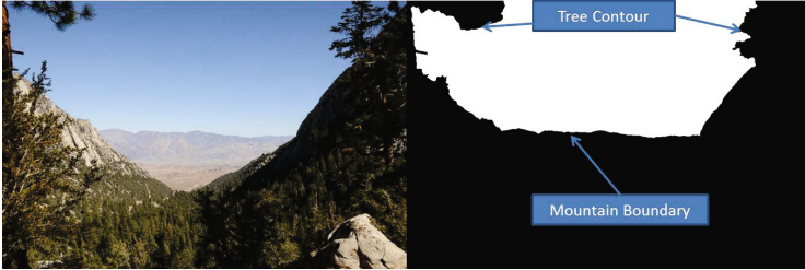
Fig. 3. Example of a query image and its skyline. The contour of the trees are false skyline pixels automatically computed from the skyline extraction model – the RANSAC-based matching process labels them correctly as outliers.
