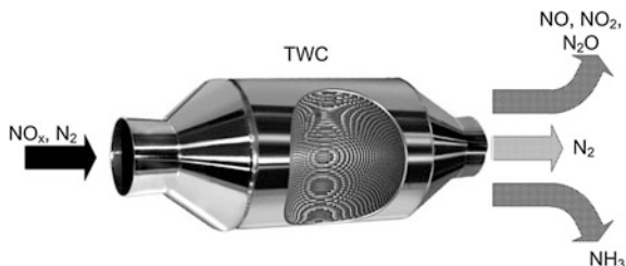
Fig. 1 Schematic of a TWC's inputs and outputs of nitrogen atoms in various chemical forms [1]
