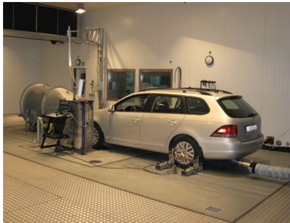
Fig. 2 Schematic overview of the exhaust emission laboratory, showing the chasis dynamometer, the climatic chamber, the various emissions measurements systems and the FTIR analyzer ( \text{NH}_3/\text{NO}_x analyser not shown)
