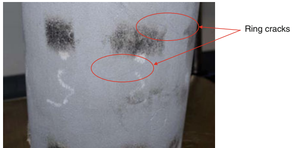
Fig. 14 SiC worst case regen, 12 g/l load with Eolys
