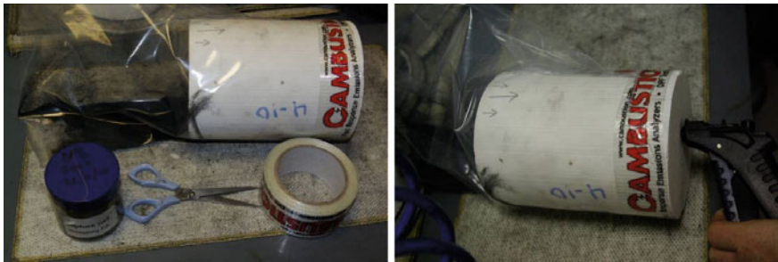
Fig. 11 Reverse aspiration of DPFs with soot aerosol
