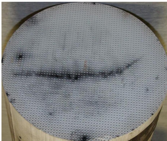
Fig. 12 Crack and missing/damaged cell plugs
