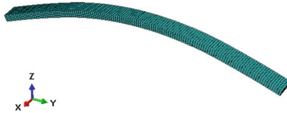
Fig. 2 Finite element mesh of the composite leaf spring
