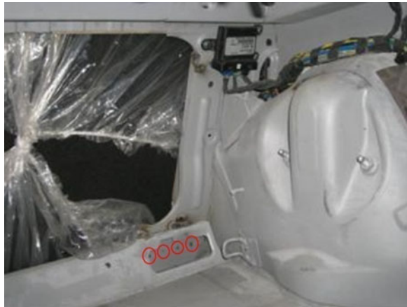
Fig. 13 Crack on spot weld of hat rack
