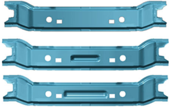
Fig. 6 The front beam parametric model in CAD
