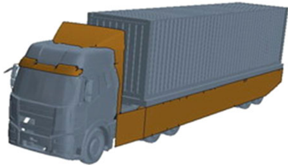
Fig. 7 Basic vehicle with deflector and side fenders (Case 2)
