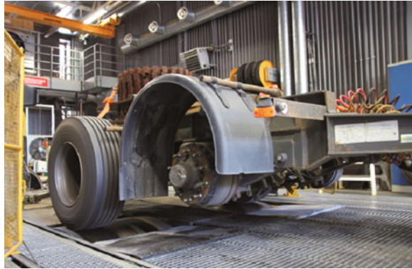
Fig. 5 Determining rolling resistance by motoring the tyres fitted on an axle of a trailer dolly
