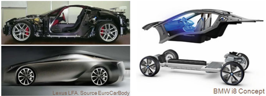
Fig. 2 Examples of vehicles that have been introduced carbon fiber parts in small series manufacturing processes
