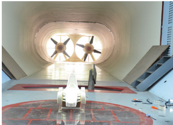
Fig. 18 Car mounted on platform balance
