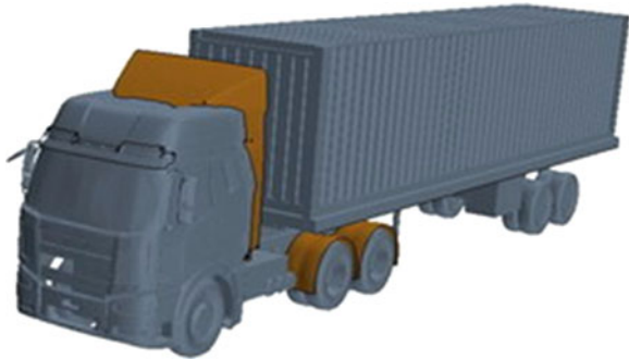
Fig. 8 Basic vehicle with deflector and without visor (Case 4)
