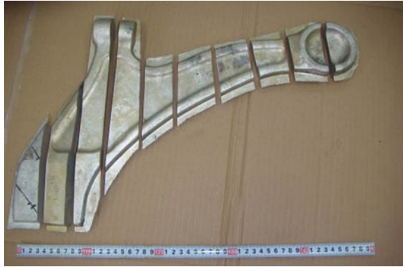
Fig. 3 The method to cut into pieces to sampling
