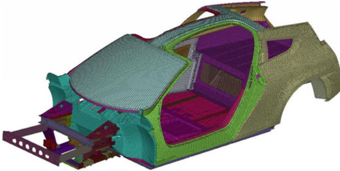
Fig. 7 Full vehicle body CAE model courtesy of delta motorsport Ltd
