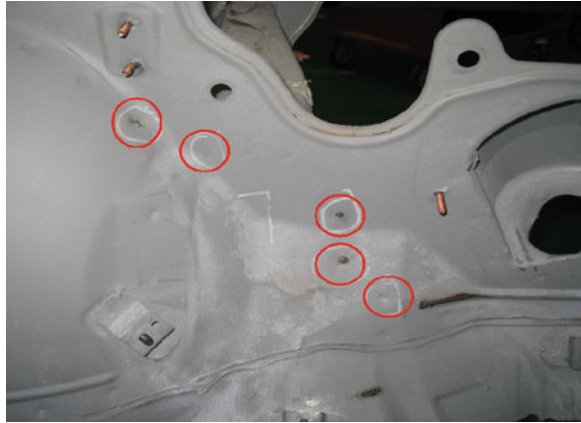
Fig. 12 Crack on spot weld of front wall
