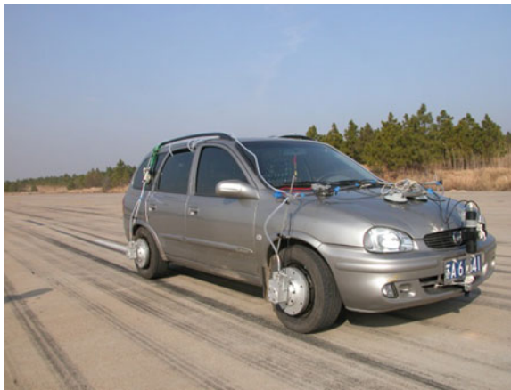
Fig. 3 The test vehicle equipped with the wheel force sensor
