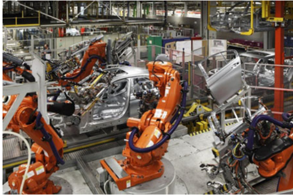
Fig. 3 BMW's highly automated production line [3]
