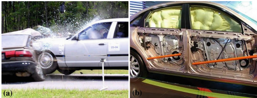
Fig. 1 a Side impact crash. b Car door with side intrusion bar installed
