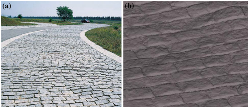
Fig. 12 a IDIADA’s pavé track b Virtual track
