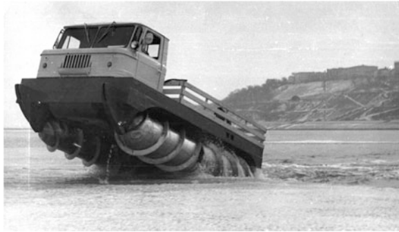
Fig. 7 Demonstration of output to the ice machine with rotary-screw mover GPI-72
