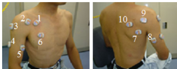
Fig. 4 Electrode placements of EMG measurement
