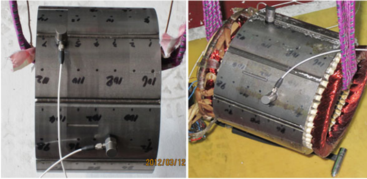
Fig. 8 Free suspension diagram of the stator with and without winding modal test
