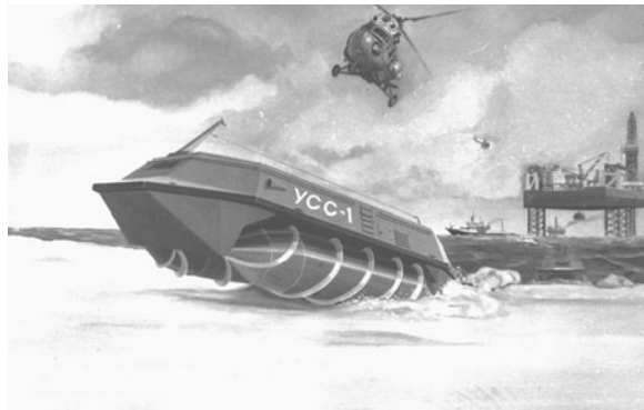
Fig. 9 Illustration of the operating conditions of the universal life-saver with rotary-screw mover
