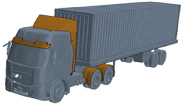
Fig. 6 Basic vehicle with deflector (Case 1)
