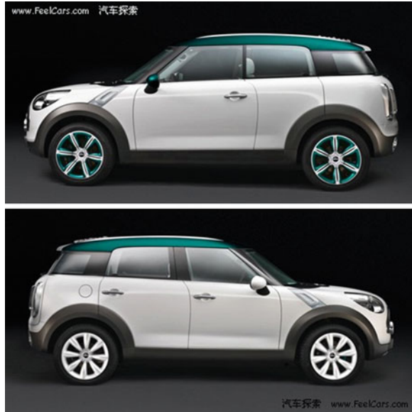
Fig. 5 The comparison of the two sides' asymmetrical design of 2008 Mini Crossover
