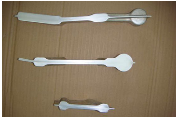
Fig. 4 Morphology of the forging sample at low magnification
