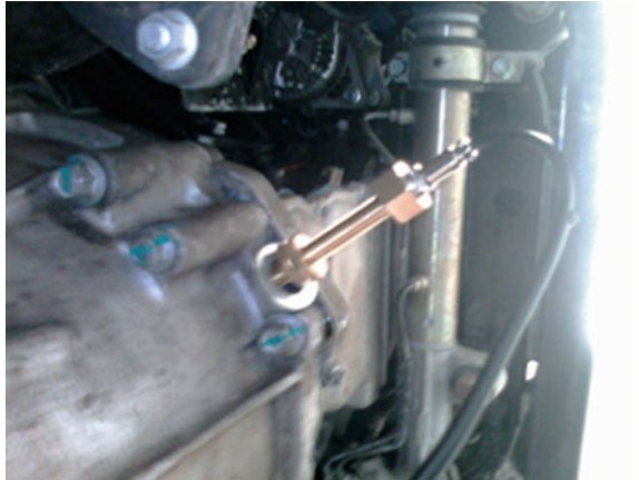
Fig. 6 Pickup at flywheel ring gear
