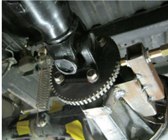
Fig. 8 Pickup at machined gear of rear axle companion flange
