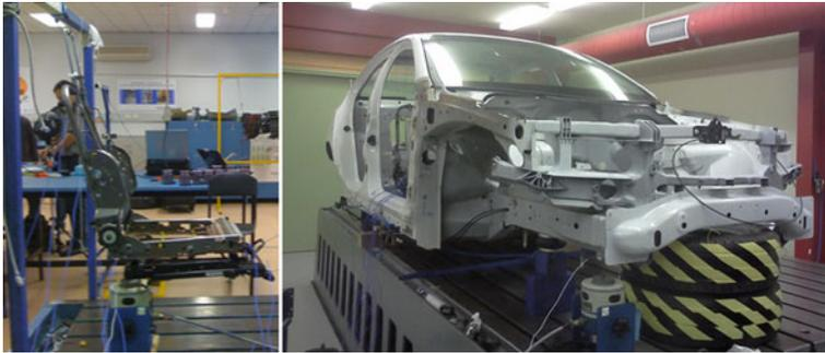
**Fig. 3** Experimental set up for BIW and seat modal testing
