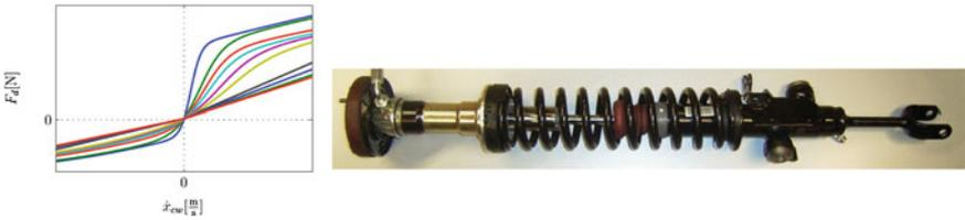
Fig. 3 Qualitative plot of the damper characteristics and realization of the hybrid suspension strut
