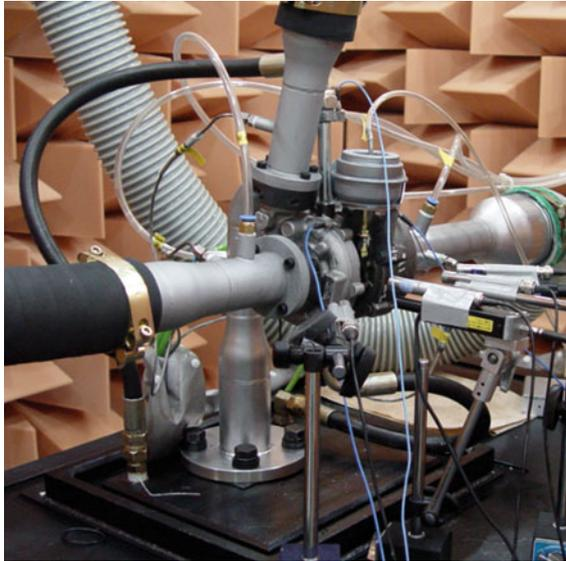
**Fig. 3** Semi-anechoic chamber for turbochargers
