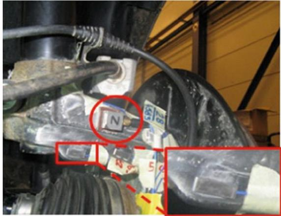
Through that, the measured indicator FRFs for inverse load-identification are not a proper representation of the actual suspension behavior in operational condition which leads to the risk of reduced load input estimation quality.
