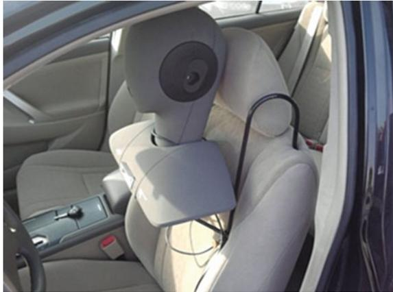
**Fig. 4** Sound quality testing spot
