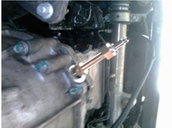
**Fig. 7** Pickup at transmission input shaft gear
