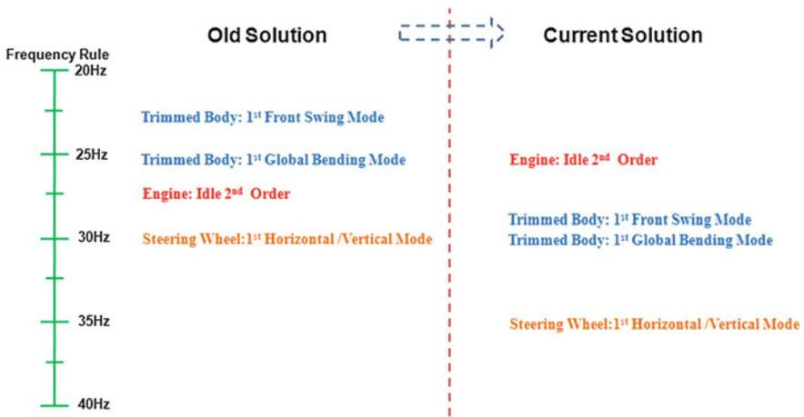
Picture 2 The mode map of main subsystem in the transfer road
