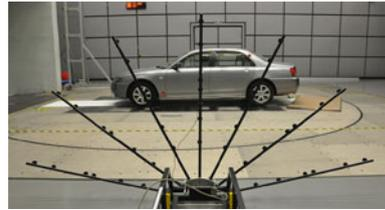
quasi-random distributions, ring-shaped, cross-shaped, linear arrays, spiral shaped etc.
