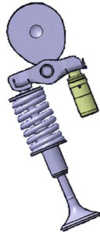
value (in this case the camshaft angle is  $20.3^\circ$ ), the valve lifter promotes the roller rocker to hit the cam, then the impact noise occurs.
