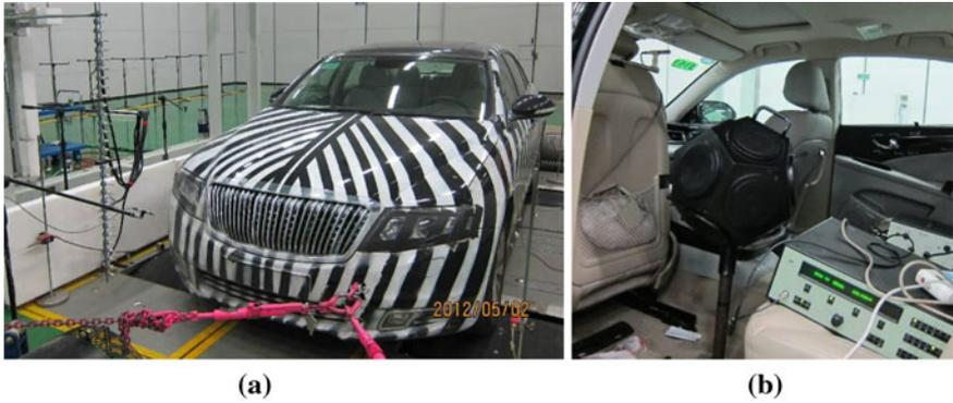
Fig. 7 The photos of test, a line array on right side of the car, b loudspeaker in the car
