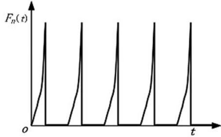
$$F_n = \begin{cases} \frac{T_e}{R}, & nT \leq t \leq (n + \frac{7}{20})T \\ 0, & (n + \frac{7}{20})T \leq t \leq (n + 1)T \end{cases} \quad (n = 0, 1, \dots) \tag{2}$$
