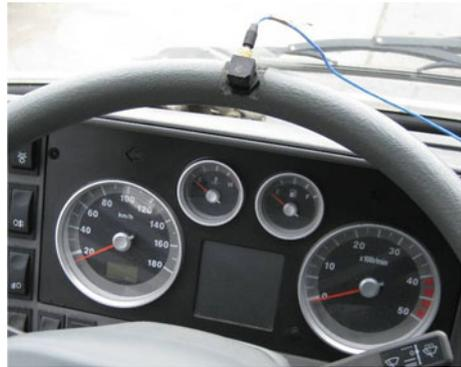
3. Installing of DVA. As shown in Fig. 11 DVA was installed in the steering wheel. The stiffness and mass were separately designed as 11000 N/m and 0.4 kg.
