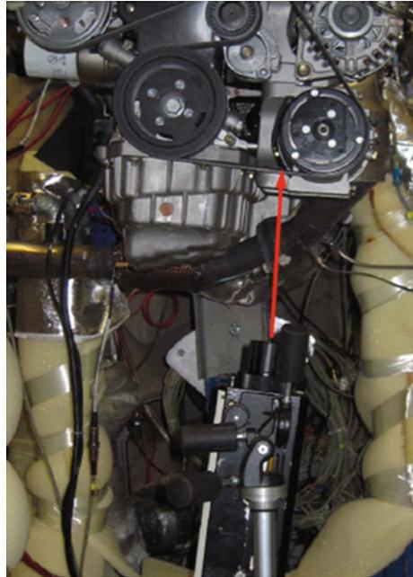
Simulation analysis of the FEAD accessory belt system was done to analyze the transverse vibration in Fig. 6, the simulation results in Fig. 7 show that the transverse vibration displacement between crankshaft pulley and AC is the greatest.
