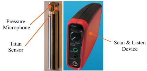
**Fig. 6** Surface microphones were used to measure surface pressure fluctuations
