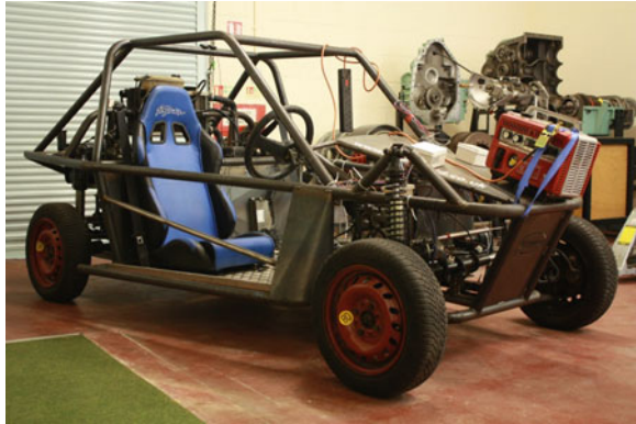
Fig. 1 The test vehicle fitted with the steer-by-wire vehicle
