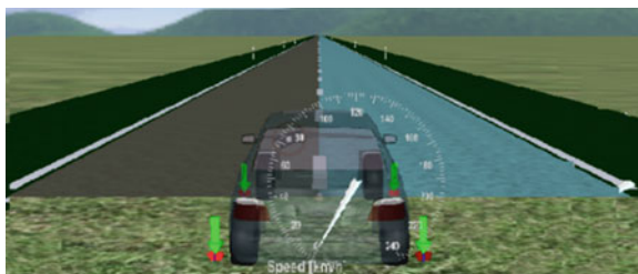
Fig. 3 A scenario of HIL simulation for braking on \mu -split road surface
