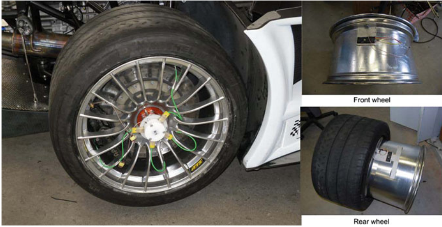
Fig. 12 Pressure and temperature sensors installed on wheels
