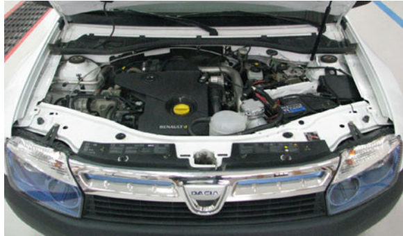
Fig. 4 The engine compartment with the auxiliary new components: the electric vacuum pump and the electric motor throttle box
