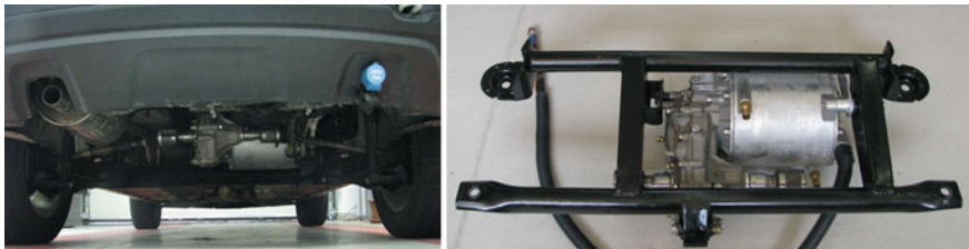
Fig. 7 The rear axle and the electric drive mounted on the frame in the rear side of the GRAND HAMSTER E 4WD
