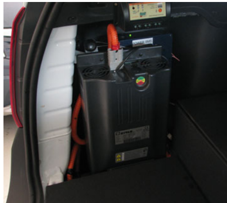
Fig. 9 The electric equipment components placed in the rear side of the vehicle: Traction battery ( in front ), the AC/DC battery charger ( vertical left ), DC/DC auxiliary battery charger ( left ); Traction Inverter Module, electric general contactor, manual connector (Anderson type) and the input energy cost meter ( right )
