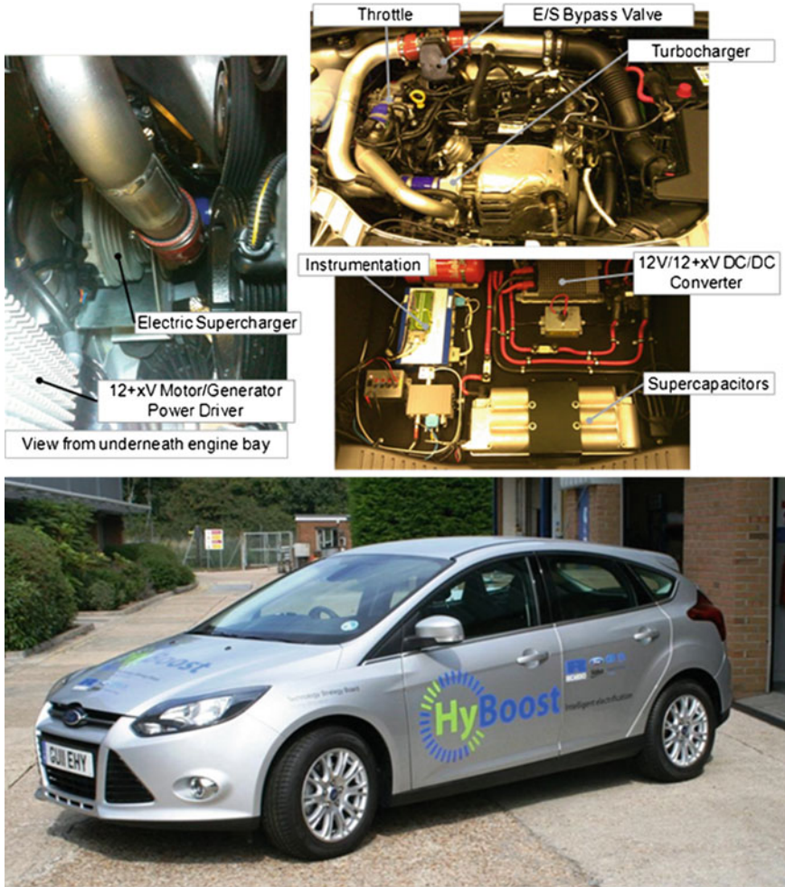
Fig. 10 HyBoost system implementation in ford focus vehicle
