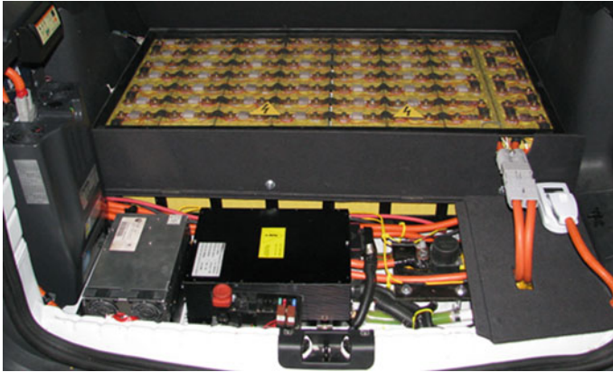
Fig. 9 The electric equipment components placed in the rear side of the vehicle: Traction battery ( in front ), the AC/DC battery charger ( vertical left ), DC/DC auxiliary battery charger ( left ); Traction Inverter Module, electric general contactor, manual connector (Anderson type) and the input energy cost meter ( right )
