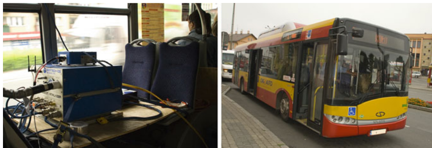
Fig. 5 View of the mounted unit's of sensors Inc. SEMTECH DS, in the vehicle with diesel engine during emission testing on route No. 0 and bus with CNG engine during testing on MPK Rzeszow bus route No. 0
