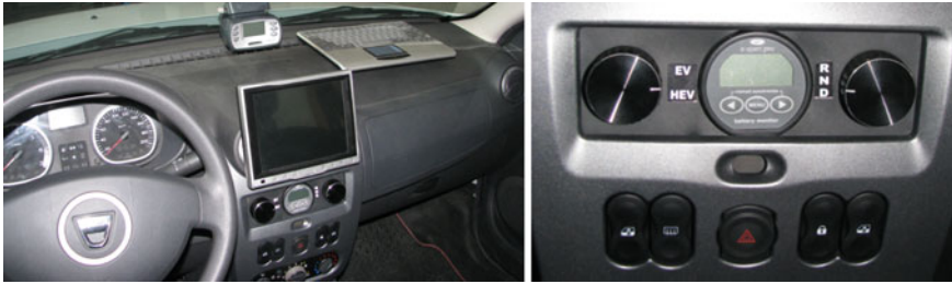
Fig. 12 The central console with the control panel of the electrical equipment: the selector button EV-HEV , the batteries monitor (traction battery and auxiliary battery) and the selector button Reverse-Neutral-Drive . Up, the PC car monitor and the VBox Raceologic display monitor
