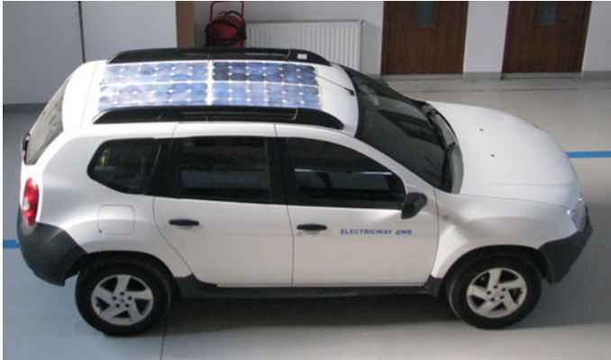
Fig. 11 The photovoltaic modules on the roof of the hybrid concept GRAND HAMSTER ELECTRICWAY 4WD
