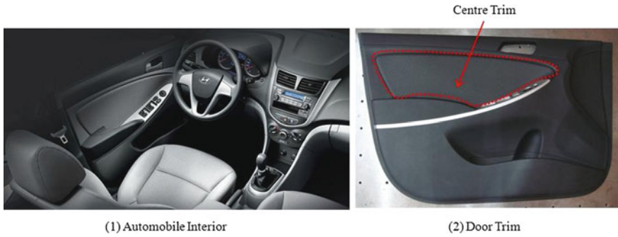
Fig. 9 The door trim and centre trim—hyundai accent. a Automobile interior, b Door trim
