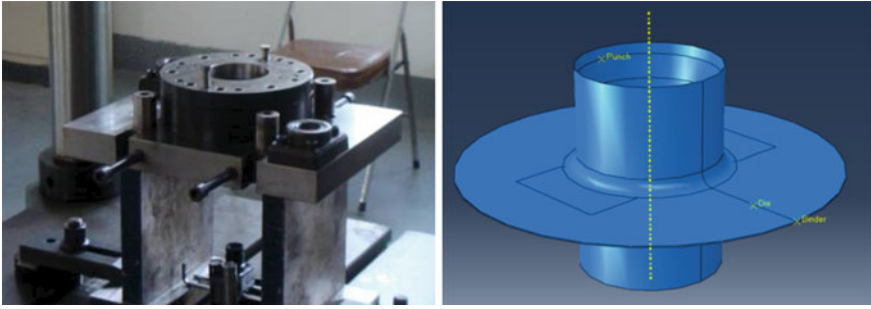
Fig. 2 The experimental apparatus and simplified FE model used for the simulation of hot metal sheet forming
