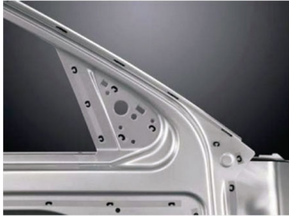
Fig. 2 Remote welding of door panel showing linear stitches and various size “C” or staple shaped welds
