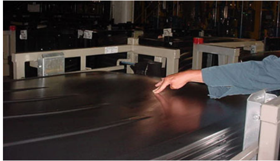
Fig. 1 Oil canning defect of truck roof
