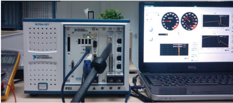
Fig. 8 PXI Real-time target, test system at global crown technology
