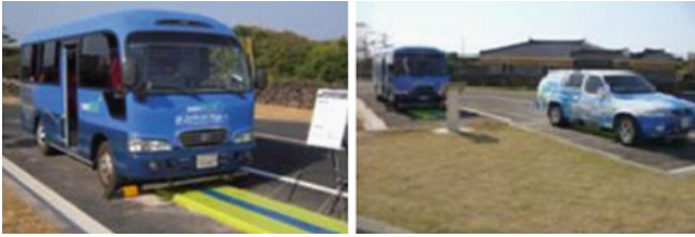
Fig. 4 KAIST stationary WPT charging system KAIST phase 1 phase 2
