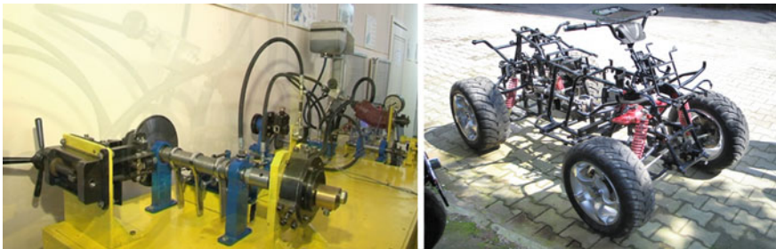
Fig. 12 The test rig and experimental vehicle to demonstrate the working principle of the Stirling alternant hydraulic propulsion system
