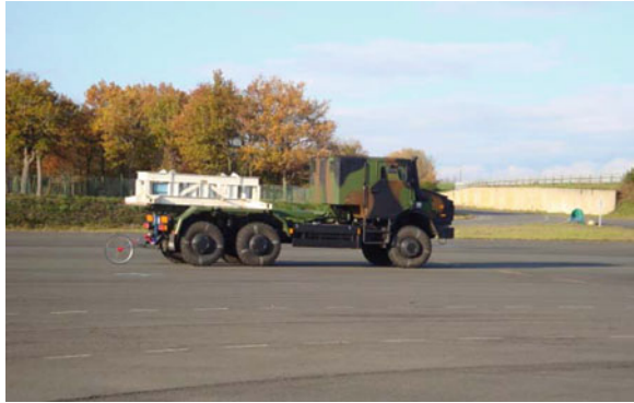
Fig. 4 Steady-state turning tests on dry and wet conditions
