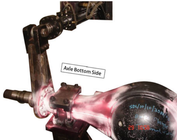
Fig. 2 Braking fatigue test setup
