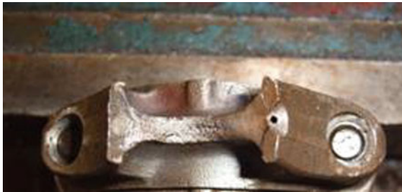
Fig. 6 Damaged location of connecting rod from experiment
