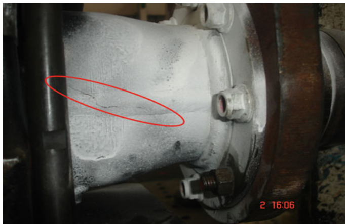
Fig. 4 Sample 1, crack observed after 261,696 cycles
