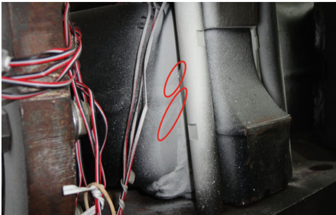
Fig. 6 Sample 3, crack observed after 136,186 cycles
