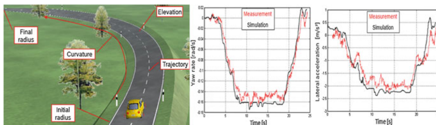
Fig. 13 Modeling of banked curves and comparison of measured and simulated quantities
