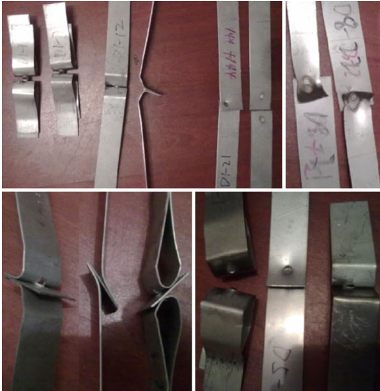
Fig. 7 Typical specimen deformation mode after test
