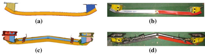
Fig. 10 Simulation and test results of head-on collision on aluminium bumper and steel a simulation result of aluminium alloy bumper, b test result of aluminium alloy bumper, c simulation result of steel bumper, d test result of steel bumper
