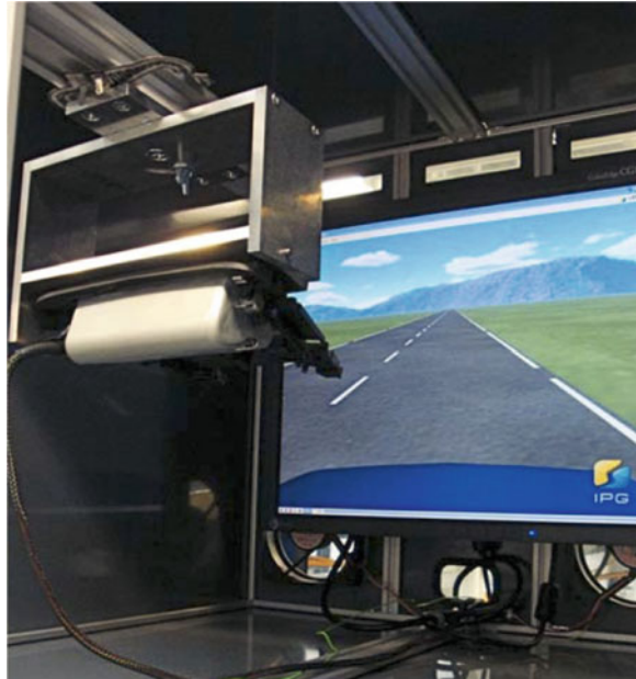
Fig. 2 Testing a LDW using a real camera
