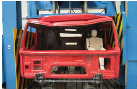
Fig. 12 Front view of the lightweight cab under top-pressure
