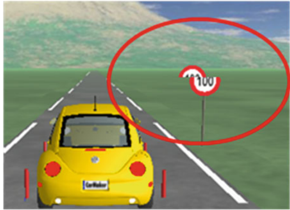
Fig. 3 Sync-delay leading to interferences
