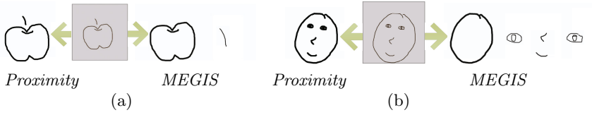
Fig. 2. Illustrations of the problems in the MEGIS algorithm. Middle column: the input sketches. Left column: segmentation results of the proposed proximity-based algorithm ( Proximity ). Right column: segmentation results of the MEGIS algorithm.
