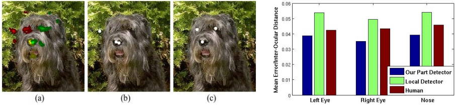
Fig. 5. An example of part detection. Left: (a) Original image overlaid with heat maps from part detectors. Red is used for the left eye, green for the right eye, and yellow for the nose; better scores are shown as brighter. (b) Detected parts using the maximum value of the detection scores. (c) Detected parts using the method described in this paper. Right: Mean localization error divided by the inter-ocular distance.
