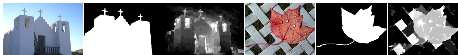
Fig. 11. Typical failure cases of geodesic saliency: (left) salient object is significantly cropped at the image boundary and identified as background; (right) small isolated background regions are identified as object
