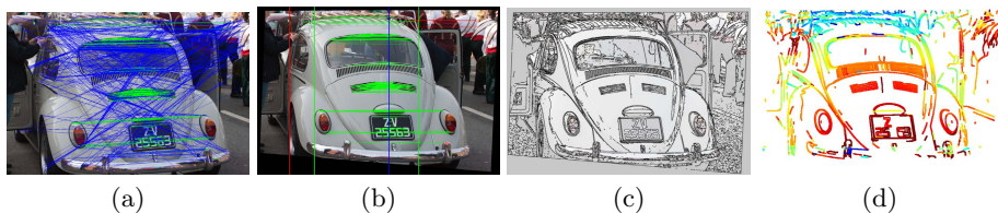
Fig. 2. Processing pipeline: (a) epipolar geometry from matched points; (b) rectified image with depth range and inlier matches (see text for a longer description); (c) extracted curves; (d) recovered depths for matched curves.
