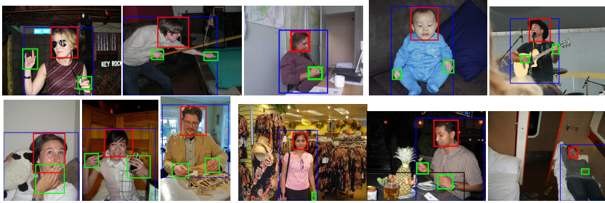
Fig. 1. Sample high ranked results of person layout detection task for the VOC 2010 test dataset. The blue rectangle represents the provided bounding box of the person, green rectangles are the detected hands and red rectangle is the detected head respectively. Our method yields the best results despite high variation in pose and occlusion.
