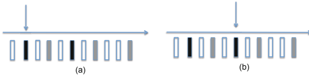
Fig. 2. Linear time constraint generation method. For a particular w the data-points with training pairs (x_i, y_i) are ordered in decreasing compatibility scores w^T \phi(x_i, y_i) (shown by the horizontal arrow sign). The vertical arrow represents the current position of the scan through the data. Gray bars are all the data-points with training pairs having the given loss value l . Black bars are the data-points with training pairs which have loss l' > l . For simplicity of the explanation, the margin is considered to be zero. In this case, a constraint is violated when a black bar is placed earlier than a gray bar in the sorted list. In (a), the first black bar will violate constraints with the three subsequent gray bars and in (b), the second black bar will violate constraints with the two remaining gray bars. If an account is maintained of all the subsequent gray bars in the list, then all the violated constraints (i, j) having \Delta_i = l can be obtained in a single scan through the data.
