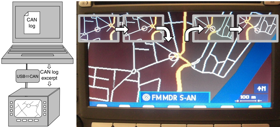
Fig. 6. Semi-automated route reconstruction – step 3: test setup and test in progress
