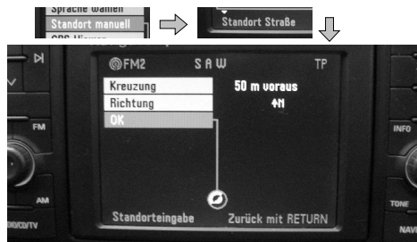
Fig. 5. Semi-automated route reconstruction – step 2 (configuring the suspected starting position)
