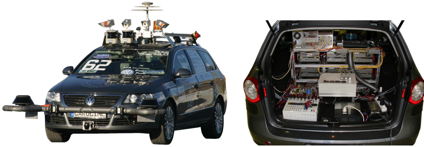
(a) Sensor setup of the autonomously driving robot vehicle “Caroline”. (b) Computers in the vehicle’s trunk, which were used to process the mass data to derive driving decisions.
