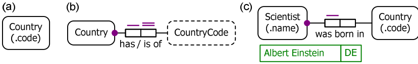
Fig. 6. A refmode in (a) compact and (b) expanded form, and (c) a populated fact type
