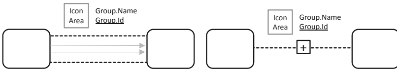
Fig. 4. Expanded and Collapsed Visual Relationship Group Shapes
