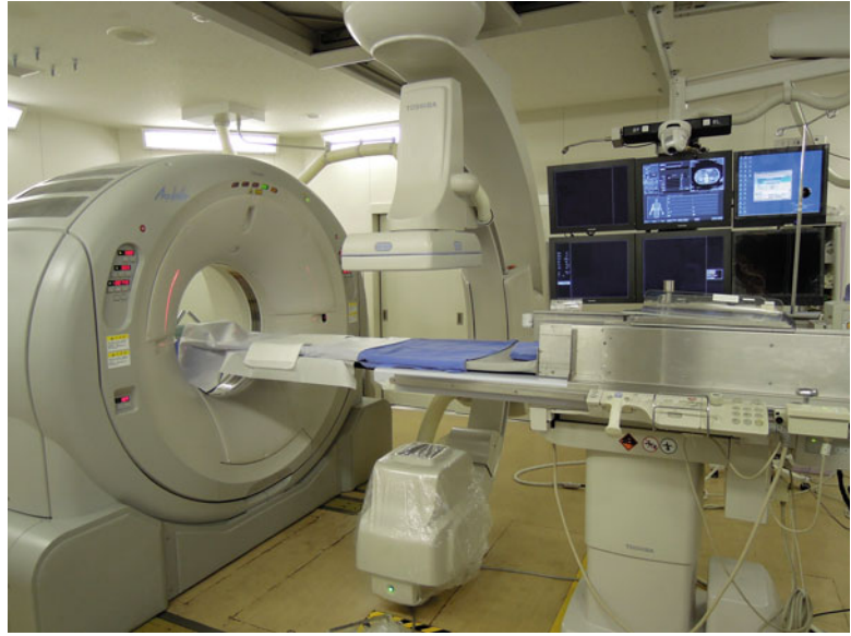
Fig. 16.20 Example of an interventional CT/angio system introduced in Nara Medical University in Japan (Infinix Activ, Toshiba Medical Systems) consisting of a CT scanner and an angio unit which are placed in line and use the same patient table
