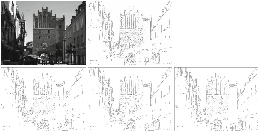
Fig. 3. Gate—input image, output of standard Canny algorithm and output of modified algorithm for \varepsilon = 10 , \varepsilon = 5 and \varepsilon = 1 respectively
