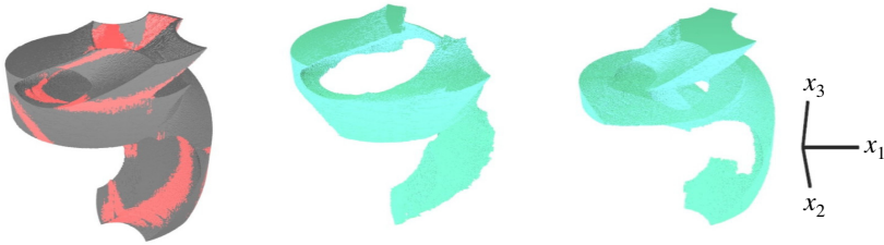
Fig. 5. Computed 3D workspace of 3-RPR (after filtering). First figure shows the undecided boxes that cover the surface of the workspace. Second and third figures show the certified connected components corresponding to the two aspects.
