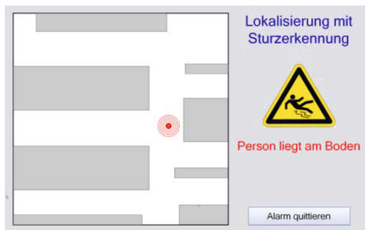
Fig. 6. Fall detection application: The name badges transmit acceleration sensor data to the system. In case of a fall, an alert is generated, indicating the location of the incident.
