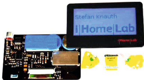
Fig. 4. Name badge with IEEE802.15.4 radio transceiver, ultrasound transmitter and LCD
