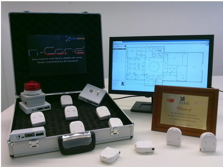
Fig. 1. n-Core Development Kit including n-Core Sirius B, Sirius D and Sirius A devices used as tags, readers and sensor controllers, respectively, in the n-Core Polaris Real-Time Locating System
