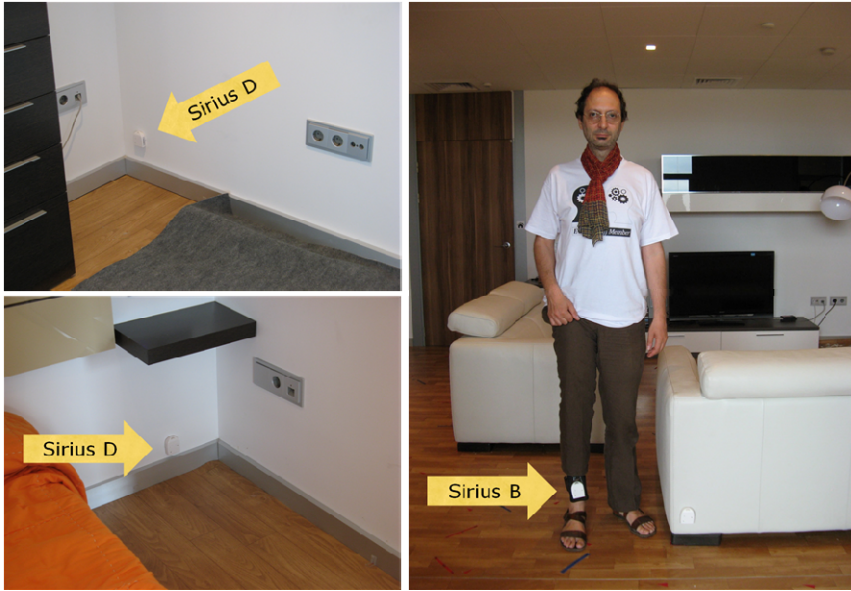
Fig. 7. Images of the deployment of the n-Core Sirius D devices used as readers and the n-Core Sirius B device used as tag during the EvAAL competition
