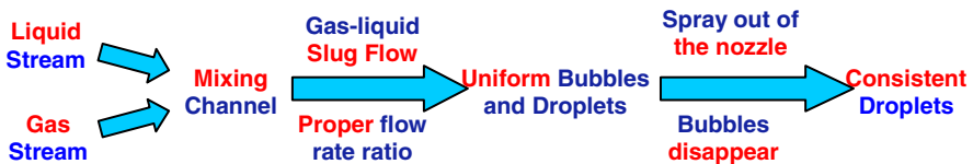
Fig. 4. The diagram of the direct driving principle for the fluid dispensing technology
