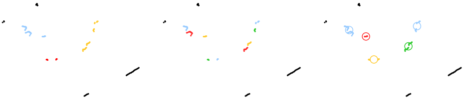
Fig. 2. Clustering approach to people detection in laser range scans. Black dots indicate points that were removed because they represent the background or are outliers. Left: Outlier and background points are removed, the remaining laser points are clustered into separate groups of people. The colors represent different group clusters. Center: Each group is clustered to roughly identify legs of people. The colors represent different leg clusters. Right: The big circles correspond to persons that result from the pairwise assignments of the legs and the remaining ones.
