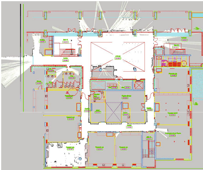
Fig. 5. Comparison of the map generated using SLAM and the building floor-plan
