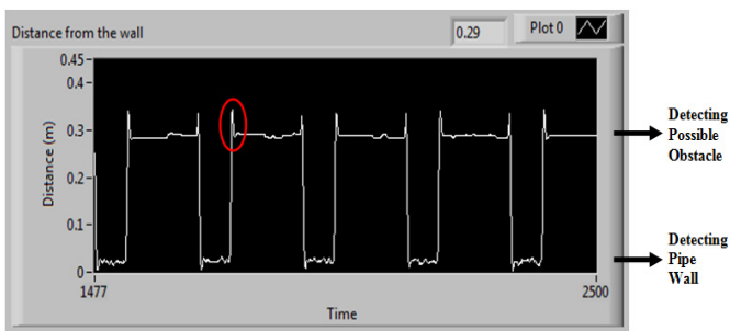
Fig. 12. Detecting obstacle and pipe wall by the sensor
