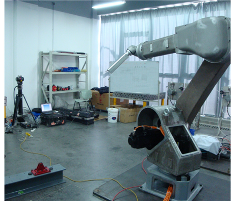
Fig. 1. The spray painting robot assembled with orientation testing tool
