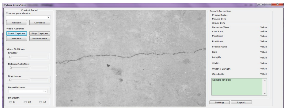
Fig. 6. User Interface of Crack Inspection System
