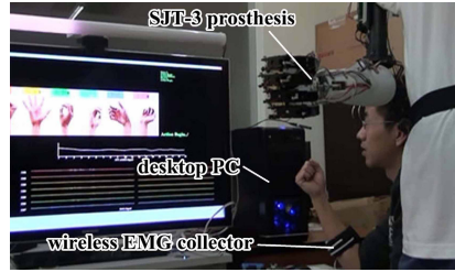
Fig. 9. Using EMG signals to control the prosthetic hand
