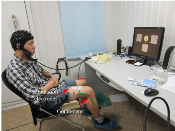
Fig. 4. Experiment Setup. The surface stimulation electrode is attached to rectus femoris, and the goniometer is to measure the knee joint angle.
