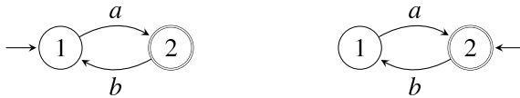
Fig. 8. SPA G (left) and DFA a \setminus G for the left quotient by the string a (right); projection P : \{a, b\}^* \rightarrow \{b\}^*
