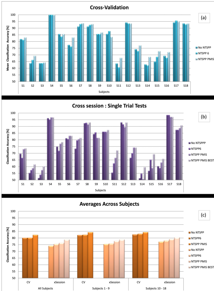
Fig. 5 BCI performance results for all subjects and approaches: (a) average cross-validation classification accuracy; (b) cross-session (x-Session) classification accuracy (c) mean accuracies across all subjects and two groups of subjects (groups based on datasets 2A and 2B). Results are presented for 3 methods: No NTSP, NTSP6 (standard embedding dimension 6 and time lag 1) and NTSP with embedding selected using PMIS and configured according to Table 3. In figures (a) and (b) the absolute best performing NTSP PMIS embedding setup is shown for information only (this best setup is the accuracy that could have been obtained if the absolute best embedding setup was determined from the training data i.e., in some cases the setup chosen did not provide the best generalization performance on the test data).
