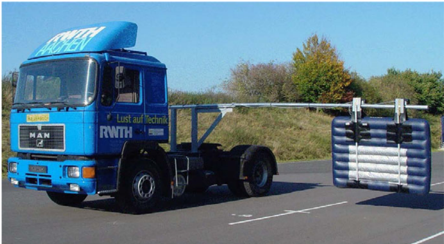
Fig. 1 Target vehicle for braking maneuvers (ika)
