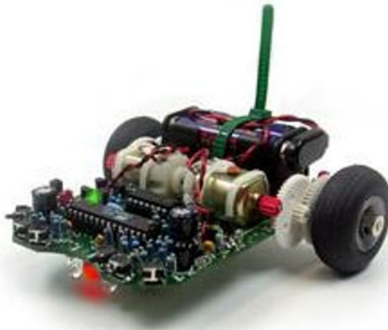
Fig. 4 “Asuro” a tiny mobile robot developed by the German Aero-Space Center (DLR)
