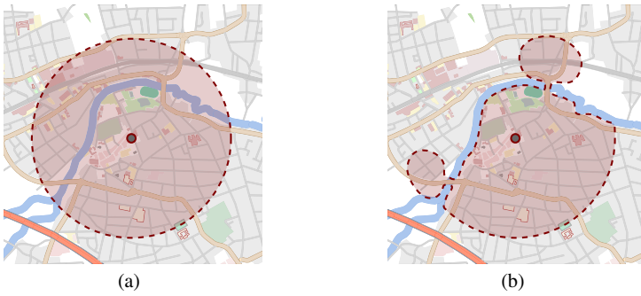
Fig. 2 The difference of a an area with distance function d_e compared to b an area with distance function d_t is particularly apparent on a poorly passable river
