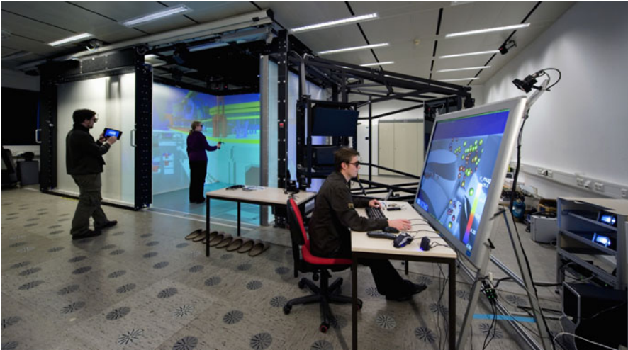
Fig. 29 Fully immersive high-end virtually reality system (CAVE) ( left ) Mid-range virtual reality system with head tracking and stereoscopic representation ( right )
