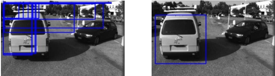
Fig. 8 Comparison between the “HaarDetectedObject” method ( left ) and the presented method ( right )
