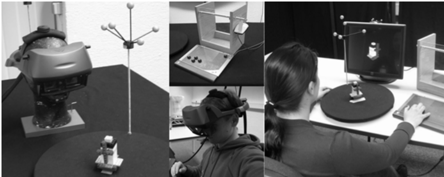
Fig. 21 Experiment configuration with turntable and HMD ( left ), experiment configuration with monitor ( right ), keypad for manipulating the virtual object ( top centre ), participant wearing the HMD ( bottom centre )
