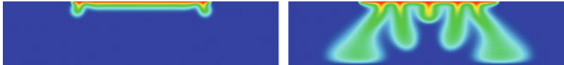
Fig. 7 Computed solution of the Elder problem in 2d at an early ( left ) and a more evolved ( right ) time point
