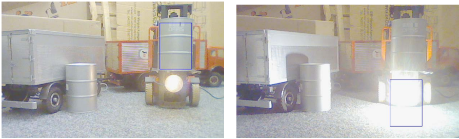
(a) Correct detection of the template (b) Matching error through the headlights of the forklift
