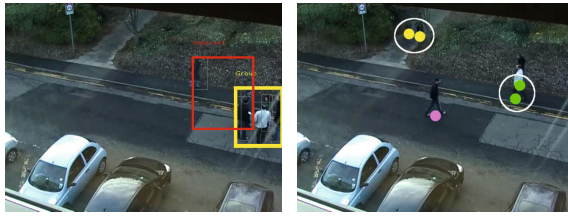
Fig. 1. Two snapshots from the BEHAVE video dataset [2]. The proposed SGT/FMTL framework recognizes the situations InGroup (yellow, thick) and concurrently Approach (red, thin) of a person (left). Mean-shift clustering results of frame 5370 (right).
